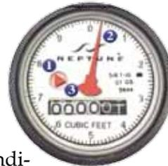
3 Meter Register – The meter register is a lot like the odometer on your car and reads straight across. The white numbers (0000) show the number of thousand of gallons that has passed through the meter.
