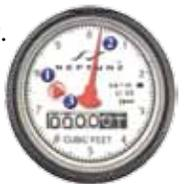
To determine if you have a leak, turn off all the water in your home, both indoor and outdoor faucets, and then check the dial for any movement of the low-flow indicator (the triangle). Movement indicates a leak.
