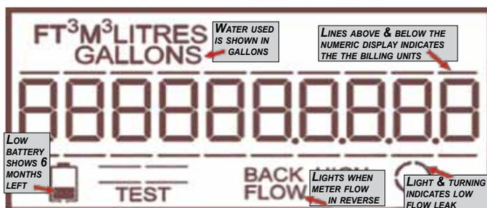
**Low-Flow Indicator** – The low flow indicator illuminates and turns if water is flowing through the meter. The numbers to the right of the decimal indicate water usage that is less than 1,000 gallons. Customers are charged for only 1,000s of gallons of water used.
