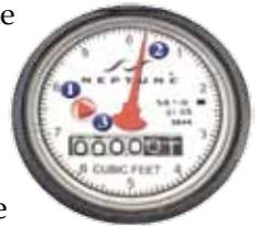
To determine if you have a leak, turn off all the water in your home, both indoor and outdoor faucets, and then check the dial for any movement of the low-flow indicator (the triangle).
